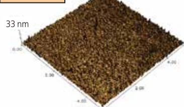
LPD層表面AFM像 AFM image of surface (LPD layer)
